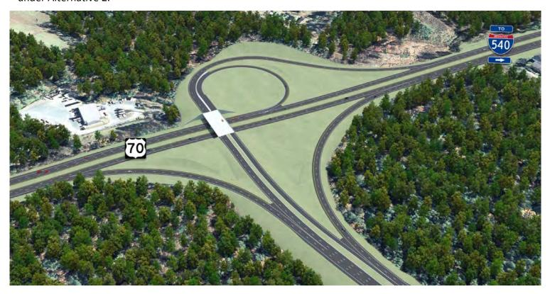
Visualization of a potential new location extension from T.W. Alexander Drive to U.S. 70, and the grade separation of U.S. 70 at T.W. Alexander Drive, under Alternative 2.
