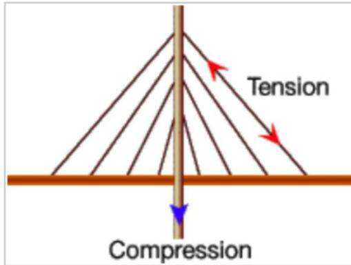
Your friend has just become an example of an "A"-Cable-Stayed suspension bridge design. This cable-stayed design, which appears to form a capital A, typically has a series of cables that branch off from the towers at different heights. The cables angle down to support the bridge deck. These cables transfer the tension back to the towers, which accommodate for the compression force on the bridge.
