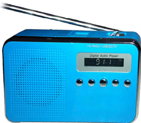
Radios with a rod antenna pick up FM signals best at a low angle or horizontal.
