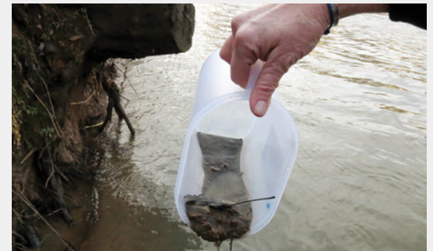
Ash separates from sediment in a scoop from the bottom of the Dan River.
