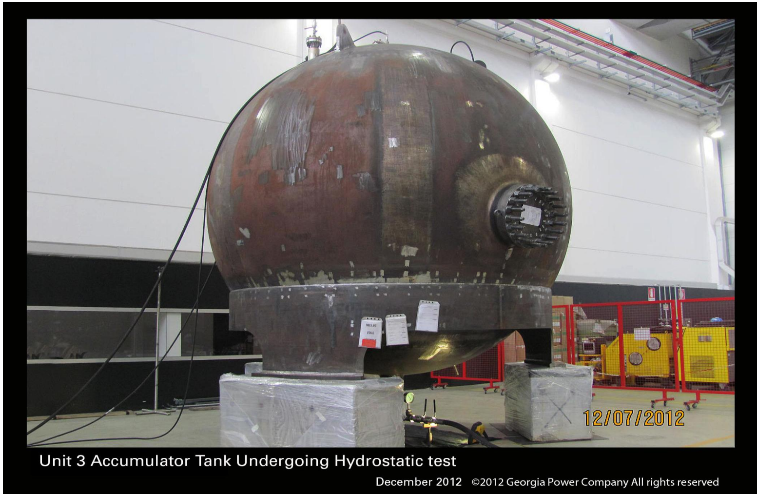
Photo 12 – Unit 3 Accumulator Tank
