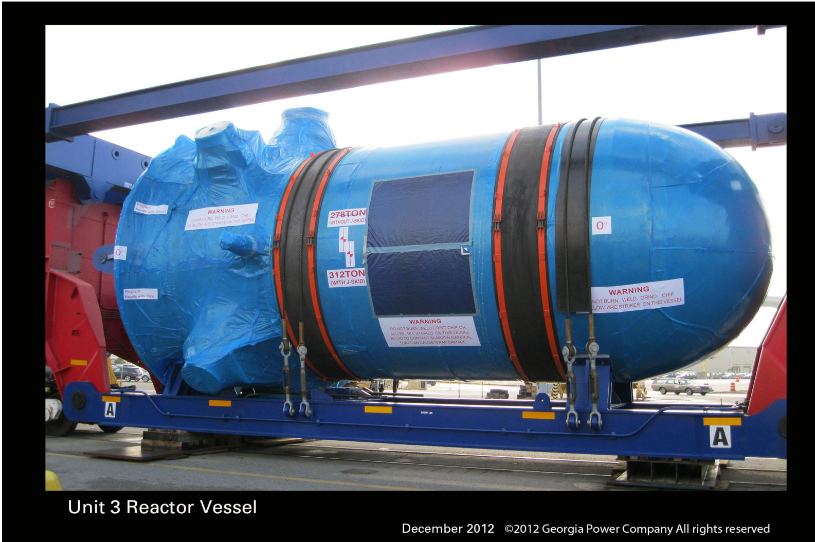
Photo 9 – Transportation of the Unit 3 Reactor Vessel
