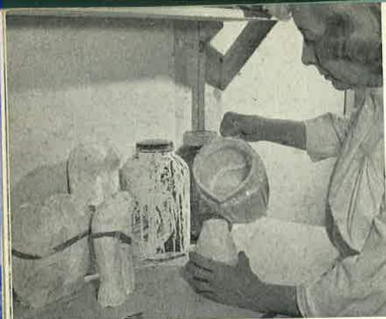
Above. From this humble beginning Dollie gets her start. The body and head are cast from plaster molds, in an unbreakable rubber compound. Successive coats of paint are applied concluding with a bisque-like washable finish in the child's own coloring.
